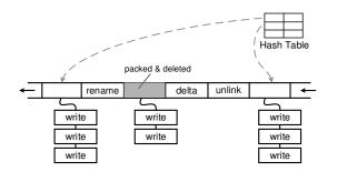
Fig. 6. Sync Queue. The nodes in Sync Queue are uploaded with a delay (e.g., 3 sec).
