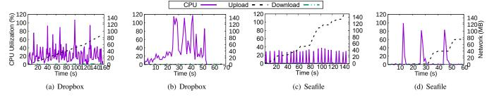
Fig. 1. Client resource consumption. (a)(c) Synchronizing a Microsoft Word file (12MB), this file is saved 23 times. (b)(d) Synchronizing a SQLite file (130MB) which stores chat history, the file is from a popular chat application. During the test, this file is modified 4 times (composed of 85 write operations) with 688KB changed in total.
