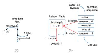
Fig. 5. **Transactional update.** (a) *Invariant of transactional update.* (b) *The procedure of executing delta encoding based on relation table.*
