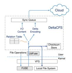
Fig. 4. DeltaCFS architecture. The grey rectangles are modules of FUSE file system.
